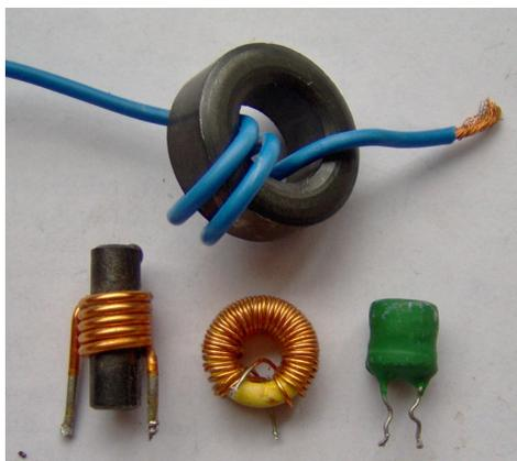
FIGURE 2.4 – Divers types de bobines. Par Miguel — Photograph, CC BY-SA 3.0, <https://commons.wikimedia.org/w/index.php?curid=1534586>
